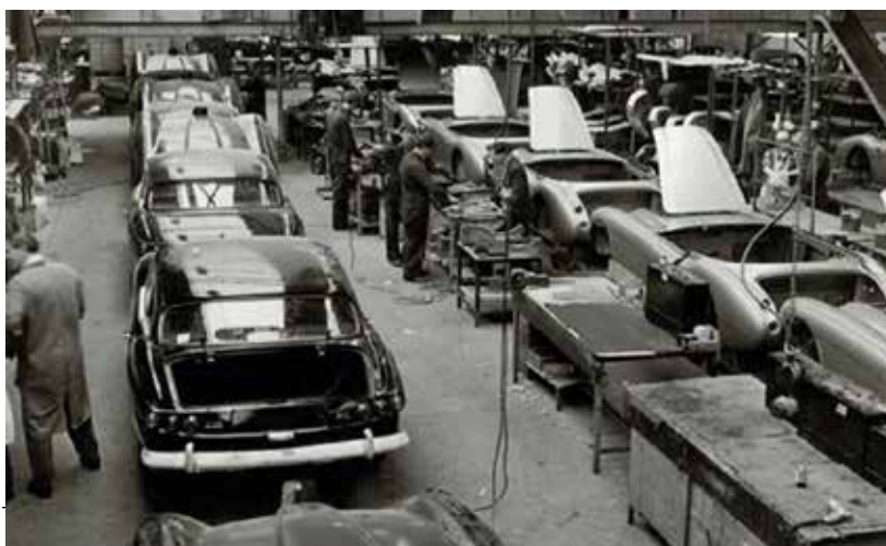
At the Jensen factory in West Bromwich. Jensen CV8s being completely assembled next to BJ8 chassis/body units.
